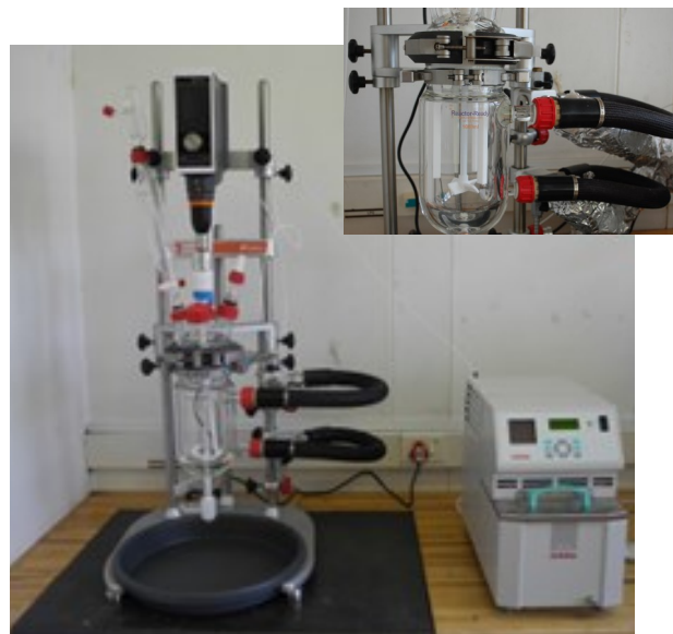
Photo: Radleys Single jacketed 1 L Process Reactor for laboratory scale up in a plant-simulated environment.
