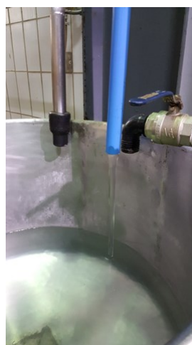
Evaporator balance tank receiving clear inulin solution exiting the ion exchange and de-colouring process
