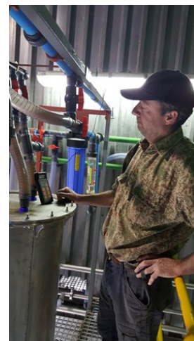
Evaporator balance tank receiving clear inulin solution exiting the ion exchange and de-colouring process
