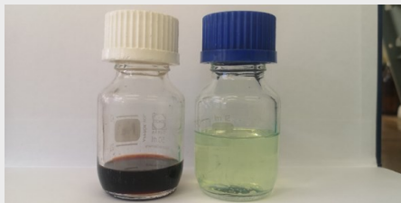
Figure 12: A-Grade Coal Hydrocracked Oil
